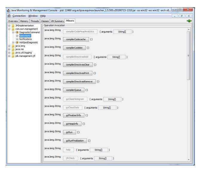
The "typical" JConsole. Operations are available under com.sun.management/DiagnosticCommand MBean.
